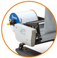
Multi-position unwind with tension control simplifies changeover
