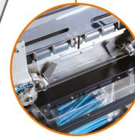
Newly designed bag sealer area combined with improved temperature control and optional seal-flatteners ensure consistent, high-quality seals
