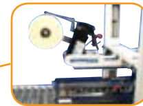
Tip-up tape head simplifies roll replacement
