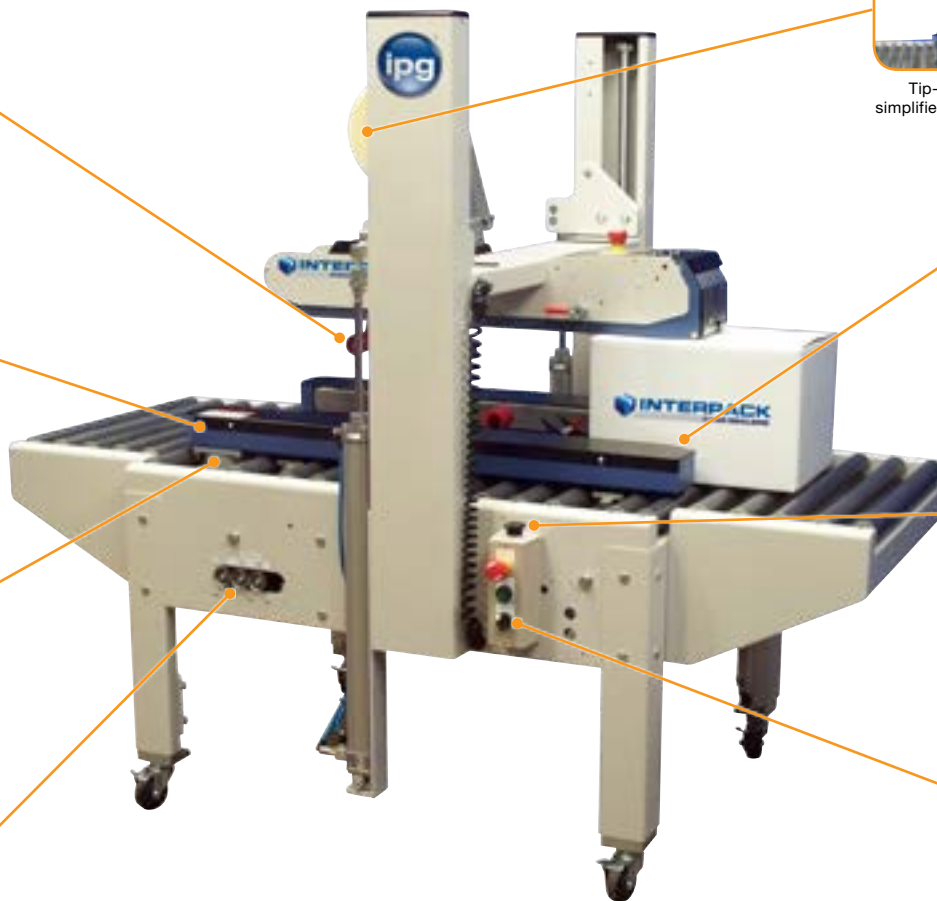
Offset tape heads process 2" high cases
