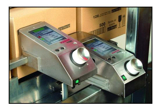
These systems can accomplish this because they are the only high resolution ink jet printers that automatically clean and maintain the printhead with a unique, patented micropurging process with every print — without affecting production speed or throughput. Unique technology builds confidence in print quality.
