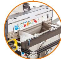
Minimal guarding provides unobstructed access to open bag
