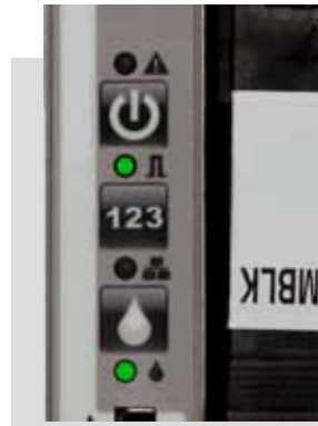
3-Logic User Interface LED indicators for intuitive use
